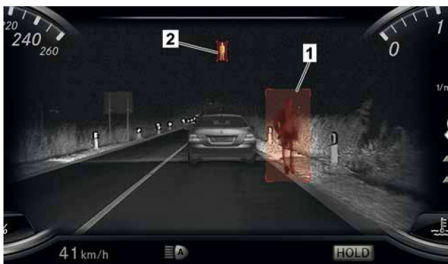
Display on instrument cluster in the dark (pedestrian detection)
