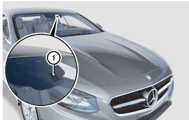
Installation location of multifunction camera
